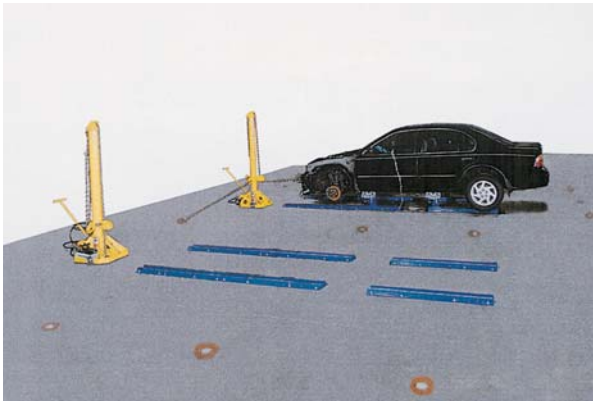
A working combination of floor tracks and anchor pots (as shown here) is another advantage when using Performance Track 2500.
